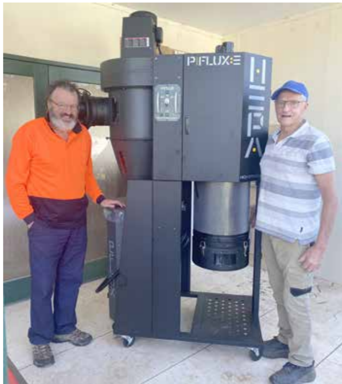
The dust extractor (yet to be installed with ductwork into the workroom, and walled in to dampen noise and prevent theft) with Aaron and Bruce proudly flanking each side.
